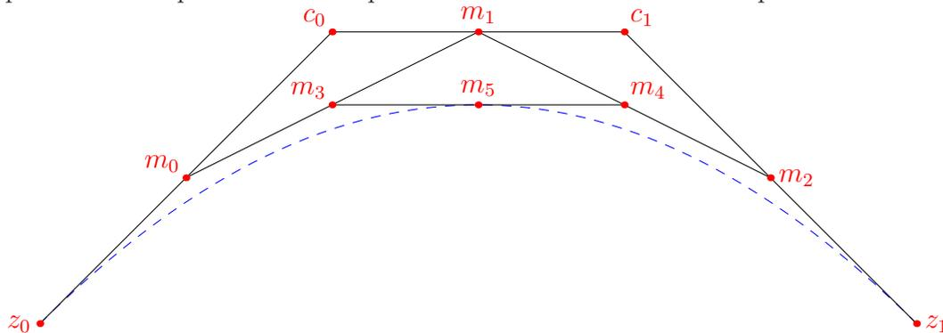
Here  $m_0$ ,  $m_1$  and  $m_2$  are the first-order midpoints,  $m_3$  and  $m_4$  are the second-order midpoints, and  $m_5$  is the third-order midpoint. The curve is then constructed by recursively applying the algorithm to  $(z_0, m_0, m_3, m_5)$  and  $(m_5, m_4, m_2, z_1)$ .
