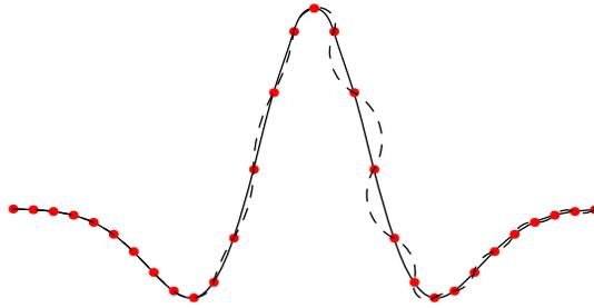
**path** a cubic spline resolved into a fixed path. In the previous example, the dashed curve is incrementally resolved at each iteration, before the entire set of nodes (shown in red) is known.
