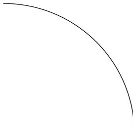
In general, a path is specified as a list of pairs (or other paths) interconnected with `--`, which denotes a straight line segment, or `..`, which denotes a cubic spline. Specifying a final node `cycle` creates a cyclic path that connects smoothly back to the initial node, as in this approximation (accurate to within 0.06%) of a unit circle:
