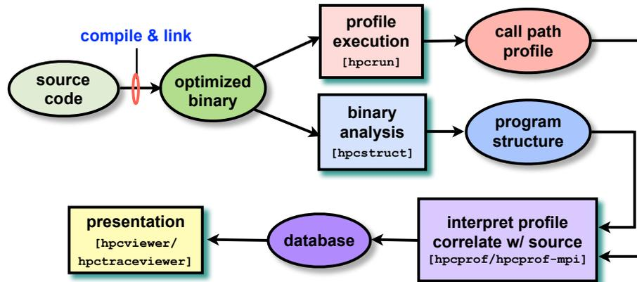
**Figure 3.1:** Overview of HPCToolkit tool’s work flow.
