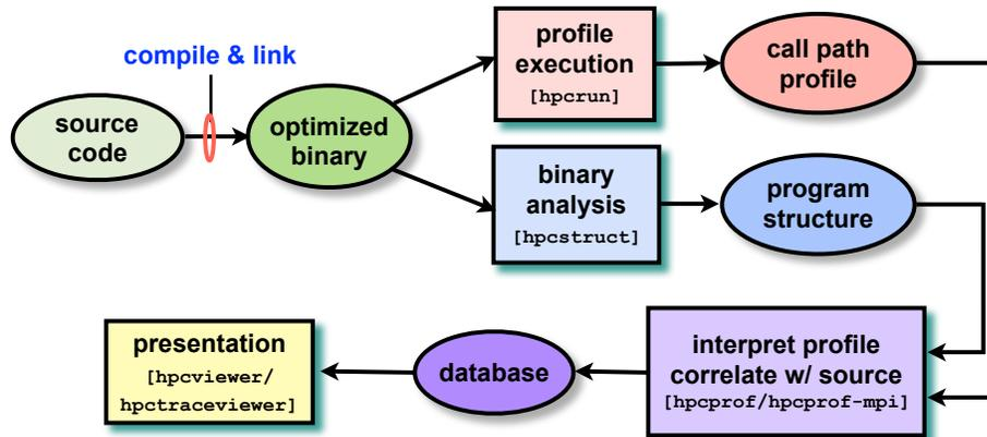
Figure 2.1: Overview of HPCToolkit’s tool work flow.
