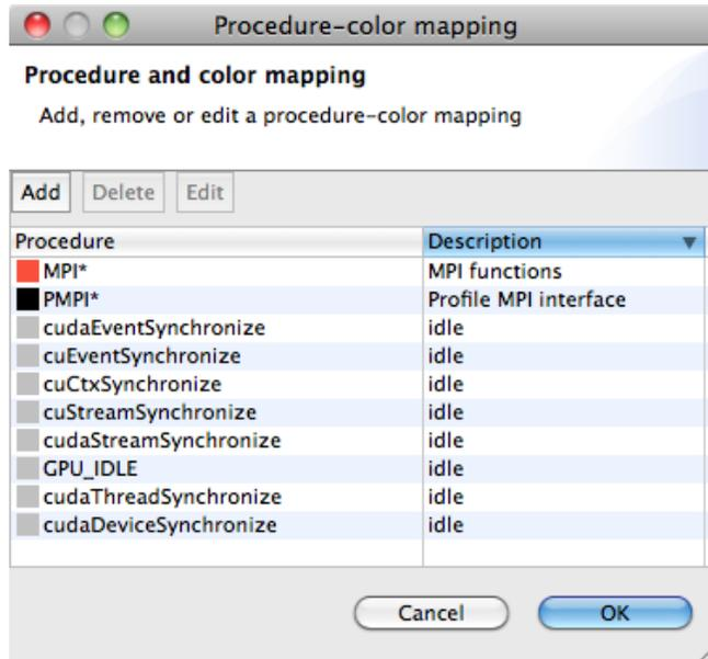
**Figure 7.4:** Procedure-color mapping dialog box. This window shows that any procedure names that match with "MPI\*" pattern are assigned with red, while procedures that match with "PMPI\*" pattern are assigned with color black.
