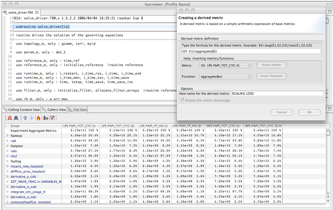
**Figure 4.6:** Computing the fraction of excess work in each program scope when applying weak scaling to go from simulating a  $30^3$  domain on one core to simulating a  $60^3$  domain on eight cores of an AMD Barcelona. The fraction of excess work is a quantitative measure of scalability loss.
