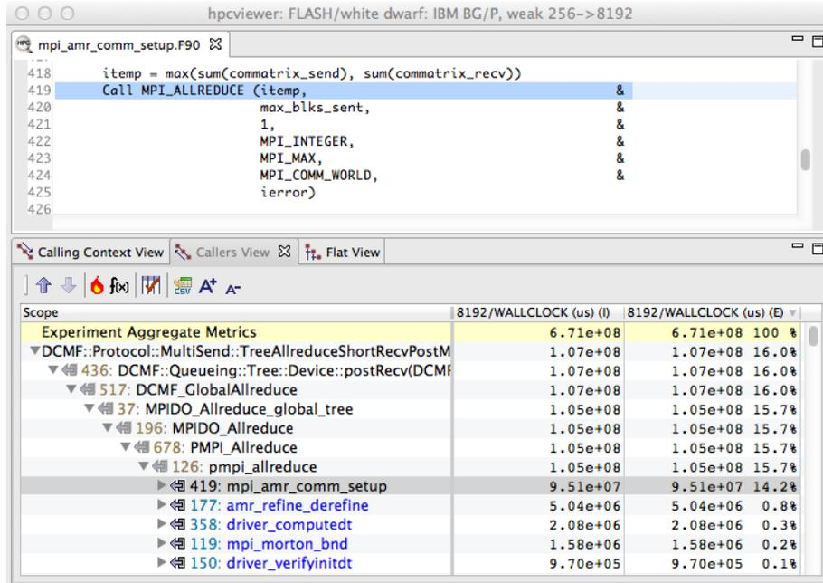
**Figure 1.1:** A code-centric view of an execution of the University of Chicago’s FLASH code executing on 8192 cores of a Blue Gene/P. This bottom-up view shows that 16% of the execution time was spent in IBM’s DCMF messaging layer. By tracking these costs up the call chain, we can see that most of this time was spent on behalf of calls to `pmpi_allreduce` on line 419 of `amr_comm_setup`.
